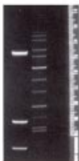
Fig. 3. High resolution of 8-48 kb size standard with asymmetric voltage FIGE.
